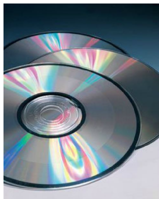
FIGURE 8.13 Diffraction of light from a compact disc. Colored interference fringes are produced by the diffraction of reflected light from the closely spaced grooves on the surface of a compact disc.
