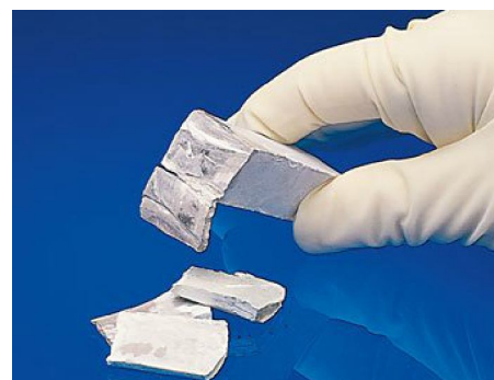
FIGURE 1.18 Sodium is a metal. The freshly exposed surface of a bar of sodium reveals its shiny metallic luster. The metal reacts quickly with moisture and oxygen to form a white coating. Sodium's high reactivity makes it dangerous to touch with bare skin.
