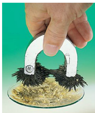
FIGURE 1.9 Formation of a mixture is a physical change. Here we see that forming the mixture has not changed the iron and sulfur into a compound of these two elements. The mixture can be separated by pulling the iron out with a magnet.
