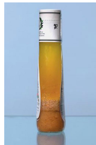
FIGURE 1.7 A heterogeneous mixture. The salad dressing shown here contains vinegar and vegetable oil (plus assorted other flavorings). Vinegar and oil do not dissolve in each other but form two layers. The mixture is heterogeneous because each of the separate phases (oil, vinegar, and other solids) has its own set of properties that differ from the properties of the other phases.
