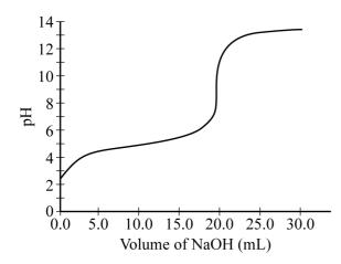
38. Data collected during the titration of a 20.0 mL sample of a 0.10 *M* solution of a monoprotic acid with a solution of NaOH of unknown concentration are plotted in the graph above. Based on the data, which of the following are the approximate  $pK_a$  of the acid and the molar concentration of the NaOH?
