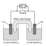
A student is given a standard galvanic cell, represented above, that has a Cu electrode and a Sn electrode. As current flows through the cell, the student determines that the Cu electrode increases in mass and the Sn electrode decreases in mass.
